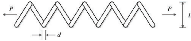
Figure 19: Schematic of tension/compression spring design
